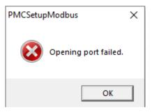
\*If error message like above appears, please check the RS-485 wiring and if the COM port is occupied by other applications
